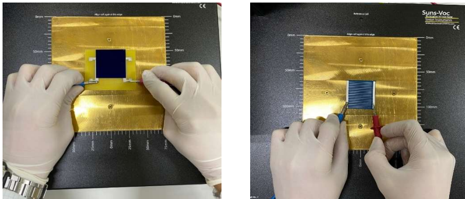
Figure 6.3 SunsVoc measurement from the front (left) and rear side (right) of the IBC solar cell
